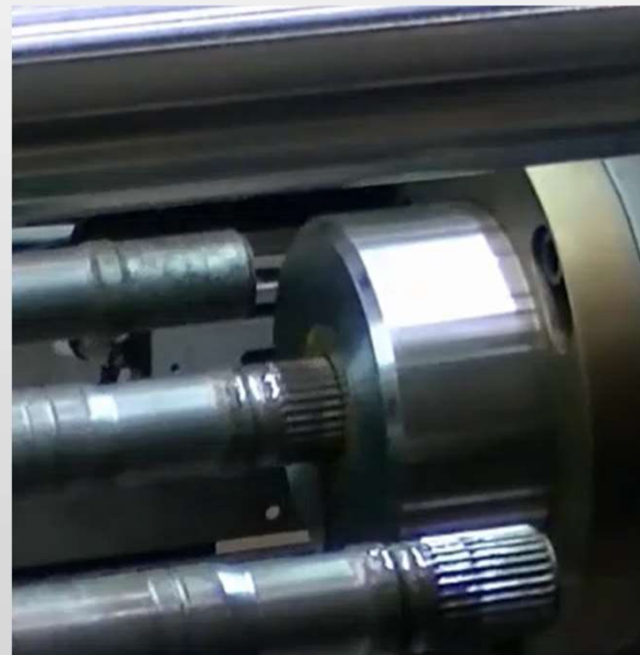
Step 2: Pulling the spline out of the die
